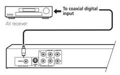
Use a coaxial cable (similar to the supplied video cable) to connect the **COAXIAL DIGITAL AUDIO OUT** jack to a coaxial input on your AV receiver.
